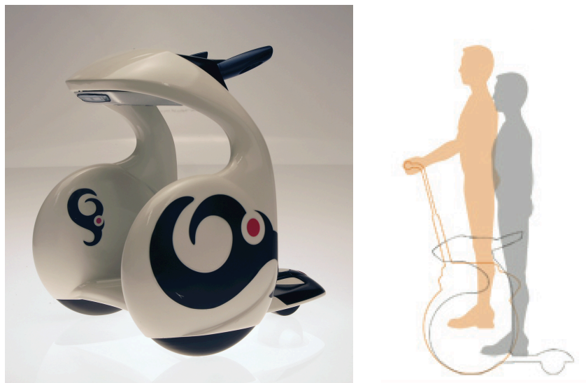
Figure 5: The final design of the GoSozo concept with personalized graphics. To the right is the GoSozo concept compared with a Segway. The occupant is lower when compared to the occupant on the Segway, which lowers the center of gravity making the device safer to use.
